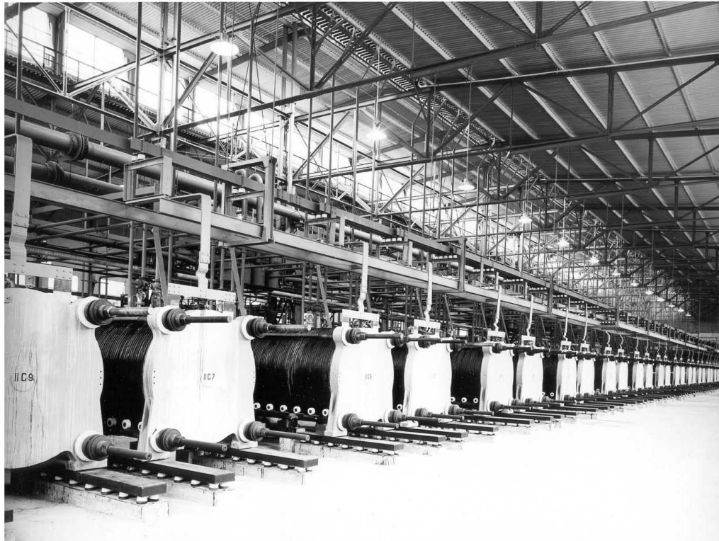
Norsk Hydro's 30,000 Nm 3 /h (~150 MW) Electrolyzer Plant (1948 - 1990)
